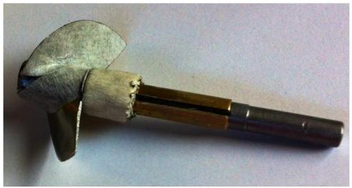
3. Mask Propeller (eg with masking tape), screws/slide onto a bolt and slide on sleeve tightly.
