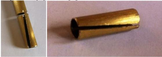
Cut slot in matching tube and cut it off (left) then
